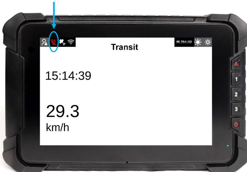
Figure 2 - Red power indicator light: device not powered
