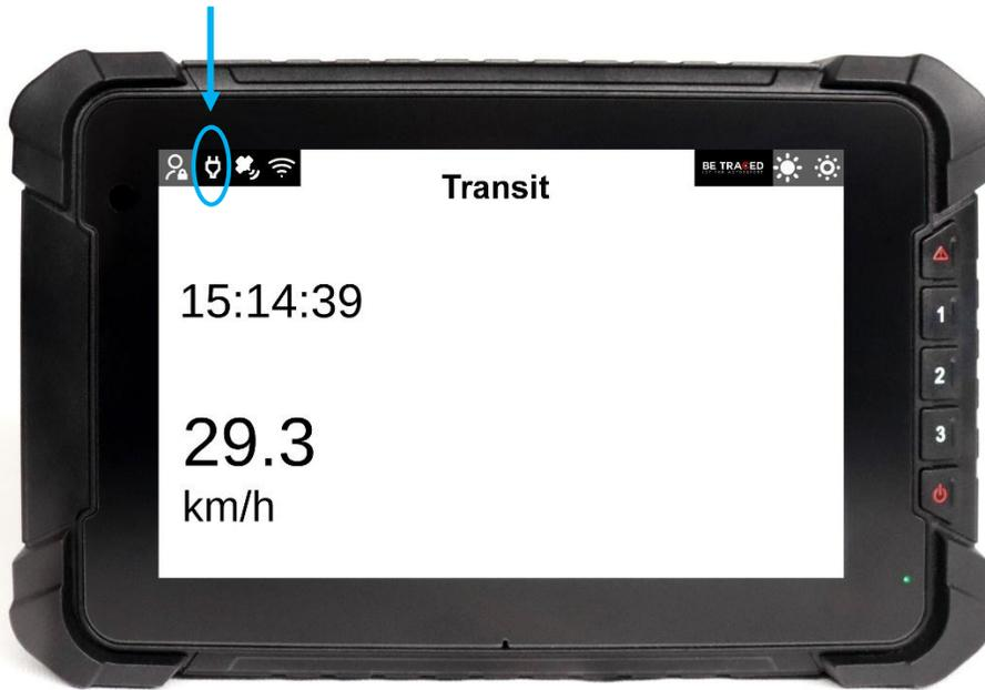
Figure 1 - White power light: device powered correctly
