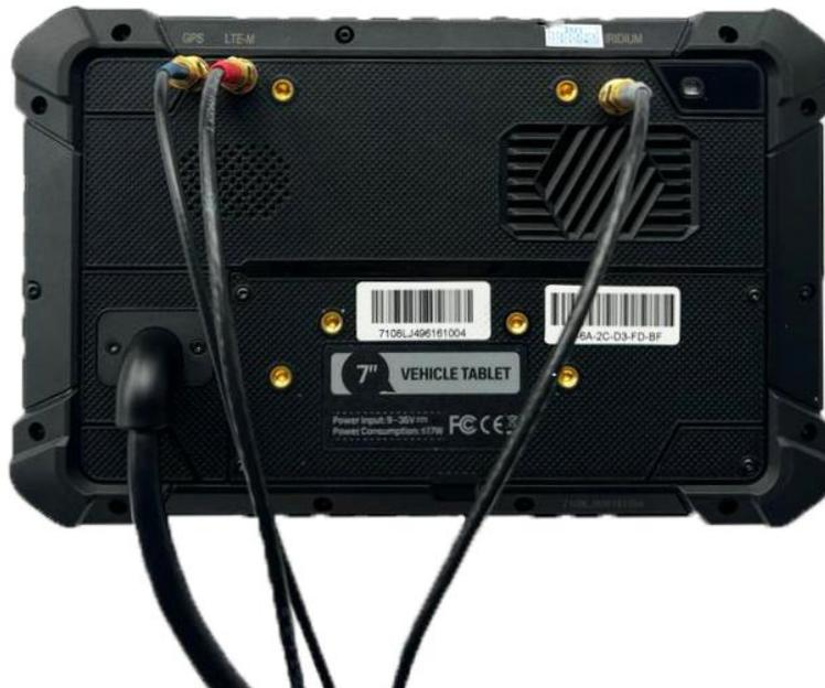
Figure 3 - Antenna connectors
